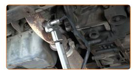
Treat the oxygen sensor connector. Use dielectric grease.
