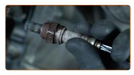
Clean the oxygen sensor mounting seat. Use WD-40 spray.
