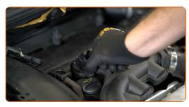
Pry up the ignition coil. Use a crowbar. Take out the ignition coil from the spark plug well.
