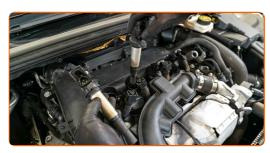
6 Clean dirt, dust and debris from inside the spark plug well.
