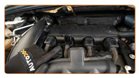
Detach the connector from the ignition coil.
