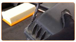
15 Reinstall the air filter housing.
