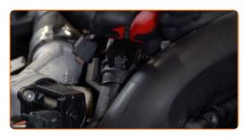
Unscrew the oil filler plug. Insert the funnel.
