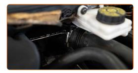
6 Disconnect the crankcase ventilation hose from the air duct.
