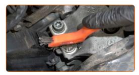
Unscrew the fasteners that connect the engine mount to the car body. Use a drive socket #E14. Use a ratchet wrench.
