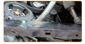
9 Return the tensioner pulley to its initial position.
