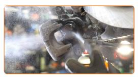
Replacement: brake pads – PEUGEOT 308 I Hatchback (4A, 4C). Tip from AUTODOC:
