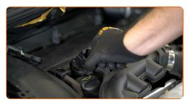
Pry up the ignition coil. Use a crowbar. Take out the ignition coil from the spark plug well.
