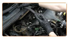
Remove the fuel filter cover with the old filter cartridge attached.
