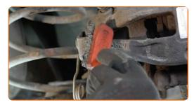
Release the parking brake cable. Use water pump pliers. Use pliers. Use a crowbar.
