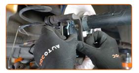
Replacement: brake pads – PEUGEOT 307 SW Box Body / Estate (3E\_, 3H\_).
