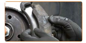
Replacement: brake pads – PEUGEOT 307 SW Box Body / Estate (3E\_, 3H\_). Tip from AUTODOC:
