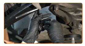
Tighten the fastener connecting the stabilizer link to the stabilizer bar. Use a drive socket #17. Use a torque wrench. Tighten it to 36 Nm torque.
