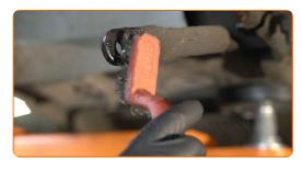
13 Install a new rod, tighten the fasteners.
