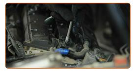
Plug in the ignition coil connector.
