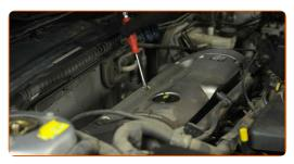
Remove the engine cover. Use a flat screwdriver.
