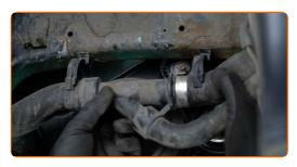
Clean the tensioner pulley fastener. Use a wire brush.
