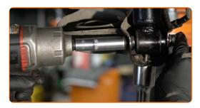
9 Remove the fastening bolt.
