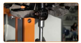
Tighten the lower fastener of the shock absorber. Use a combination spanner #13. Use a drive socket #15. Use a torque wrench. Tighten it to 57 Nm torque.
