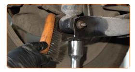
Unscrew the lower fastener of the shock absorber. Use a combination spanner #13. Use a drive socket #15. Use a ratchet wrench.
