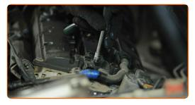
Plug in the ignition coil connector.
