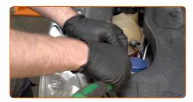
Remove the coolant reservoir cap.
