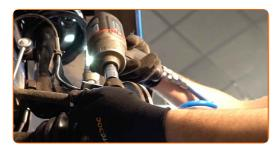
Disconnect the tie rod end from the steering knuckle. Use a pin punch. Use a hammer.
