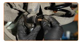
Tighten the lower fastener of the shock absorber. Use a combination spanner #13. Use a drive socket #15. Use a torque wrench. Tighten it to 57 Nm torque.
