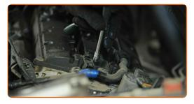
Plug in the ignition coil connector.
