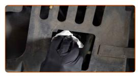
Screw in the new drainage plug and tighten it. Use HEX No.H8. Use a torque wrench. Tighten it to 30 Nm torque.
