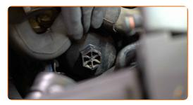
Unscrew the filter housing cap together with the old filter element. Use a drive socket #27.
