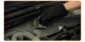
Tighten the oil filler cap.
