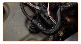
Remove the crankcase ventilation hoses.
