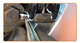
Install the retaining springs of the brake pads.
