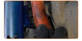
Unscrew the fastener connecting the stabilizer link to the shock strut. Use a drive socket #17. Use a ratchet wrench.
