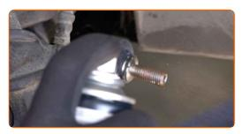
Install a new stabiliser link and tighten the fasteners. Use a drive socket #17. Use a ratchet wrench.
