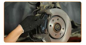
Replacement: brake pads – PEUGEOT 306 Hatchback. Tip:
