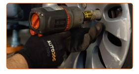
Lower the car and working in a cross order, tighten the wheel bolts. Use a torque wrench. Tighten it to 100 Nm torque.
