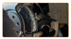
Install the brake caliper and fix it. Use a combination spanner #13. Use a combination spanner #15. Use a torque wrench. Tighten it to 27 Nm torque.
