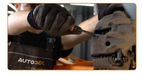
10 Remove the brake caliper.
