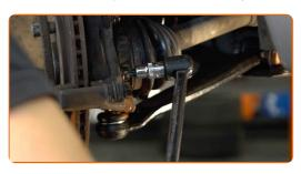
Remove the caliper bracket.
