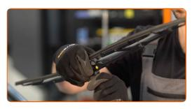
Remove the blade from the wiper arm.
