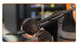
Remove the blade from the wiper arm.
