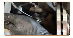
Screw on the fastening nut that connects the tie rod end to the steering knuckle. Use a drive socket #17. Use a ratchet wrench.
