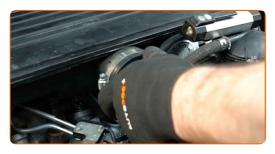
Screw in the air hose clamps. Use a drive socket #7. Use a ratchet wrench.
