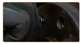
Tighten the brake disc fasteners. Use Torx T30. Use a torque wrench. Tighten it to 10 Nm torque.
