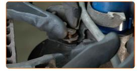
Tighten the brake hose fastening bracket to the shock strut. Use a drive socket #13. Use a torque wrench. Tighten it to 12 nm torque.
