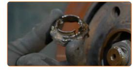
Loosen the fastener of the driveshaft. Use a drive socket #36. Use a tap wrench.
