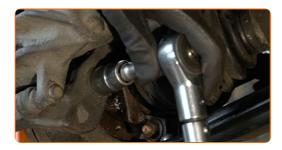
79 Install the brake hose bracket.
