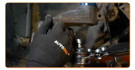
Fix the shock absorber strut on the steering knuckle.
