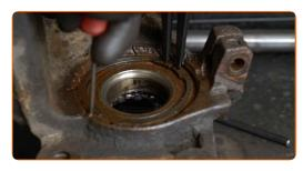
Dismantle the inner bearing race that is remaining on the hub. Bush and bearing driver set. Use a bearing separator.
