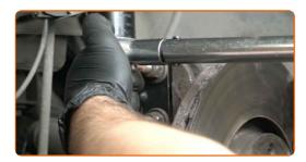
Tighten the drive shaft nut. Use a drive socket #36. Use a torque wrench. Tighten it to 280 Nm torque.
