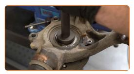
Pull the bearing inner race out of the wheel hub. Use a bearing separator. Use 3-Arm Gear Puller.
