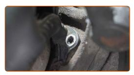
Tighten the fastener that connects the ABS sensor to the steering knuckle. Use a drive socket #10. Use a torque wrench. Tighten it to 11 nm torque.
