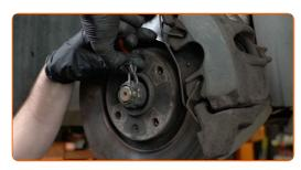
Clean the fastener of the driveshaft. Use a wire brush. Use WD-40 spray.
