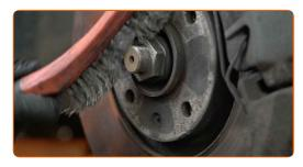
Loosen the fastener of the driveshaft. Use a drive socket #36. Use a ratchet wrench.
