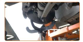
Disconnect the spherical joint from the arm. Use a crowbar.
