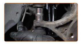
Fix the shock absorber strut on the steering knuckle. Use a crowbar.
