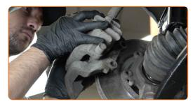
Tighten the brake caliper bracket. Use Torx T50. Use a torque wrench. Tighten it to 105 Nm torque.
