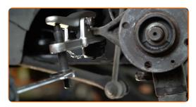
Unscrew the lower fastener connecting the shock strut to the steering knuckle. Use a combination spanner #18. Use a drive socket #18. Use a ratchet wrench.
