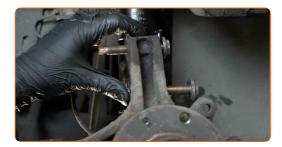
Clean the ABS sensor fastener. Use a wire brush. Use WD-40 spray.
