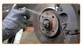
70 Clean the brake disk surface. Use a brake cleaner.
