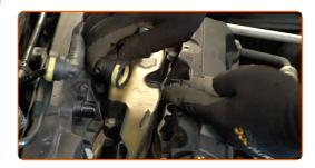
Detach the connector from the ignition coil.
