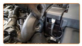
Connect the vacuum sensor. Squeeze the clamp with combination pliers and connect the vacuum valve hose.
