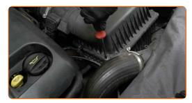
A Slightly raise the cover of the air filter housing.
