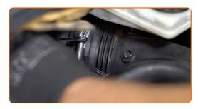
Connect the charger intake hose to the air filter housing.
