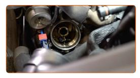
Screw the new filter into its place.
