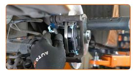
Install the brake caliper and fix it. Use a combination spanner #19. Use a drive socket #13. Use a torque wrench. Tighten it to 30 Nm torque.
