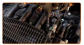
**14** Treat the ignition coil connector with electronic spray. The spray will protect the electrical contacts from corrosion, oxidation, and will reduce the contact resistance.
