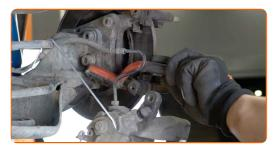
Unscrew the caliper bracket fastening. Use Torx T55. Use a tap wrench.
