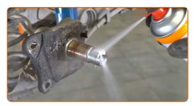
Treat the stub axle. Use a multipurpose grease. Use a flat screwdriver.
