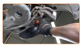
28 Install the brake caliper bracket.
