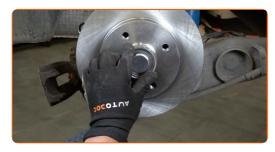
Clean the mounting seats of the caliper and its bracket. Use a wire brush. Use WD-40 spray.
