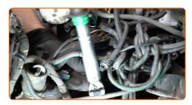
Tighten the thermostat housing mounting stud. Use a drive socket #E5. Use a torque wrench. Tighten it to 11 nm torque.
