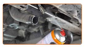
Attach the lower coolant pipe.
