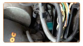
Install the engine wiring harness cover. Make sure you hear a click indicating that it is locked in place.
