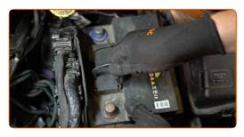
Attach the terminals to the battery.
