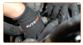
Secure the coolant hose clamp. Use a drive socket #7. Use a ratchet wrench.
