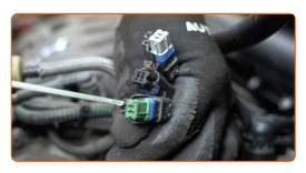
Attach the engine wiring harness connectors.
