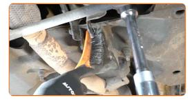
12 Install the engine mount to its mounting seat.
