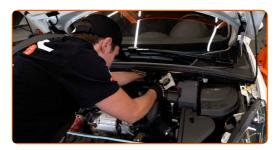
Screw in the fastening screws of the air filter cover (3 pieces). Use Torx T25. Use a ratchet wrench.
