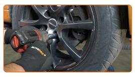
Lower the car and working in a cross order, tighten the wheel bolts. Use wheel impact socket #17. Use a torque wrench. Tighten it to 100 nm torque.
