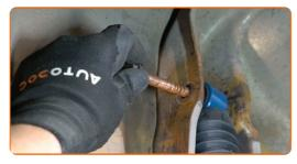
Screw the upper fastener of the shock absorber. Use a combination spanner #16. Use a drive socket #16. Use a ratchet wrench.
