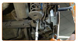
Tighten the top shock absorber fastening. Use a drive socket #16. Use a torque wrench. Tighten it to 60 Nm torque.
