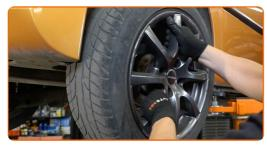
Remove the plastic clips of the wheel arch liner. Use a clip removal tool.
