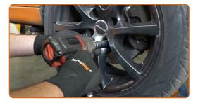
Lower the car and working in a cross order, tighten the wheel bolts. Use wheel impact socket #17. Use a torque wrench. Tighten it to 100 nm torque.
