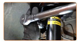
Tighten the fastener connecting the stabilizer link to the stabilizer bar. Use a drive socket #17. Use a torque wrench. Tighten it to 43 Nm torque.
