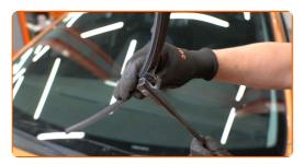
Remove the blade from the wiper arm.
